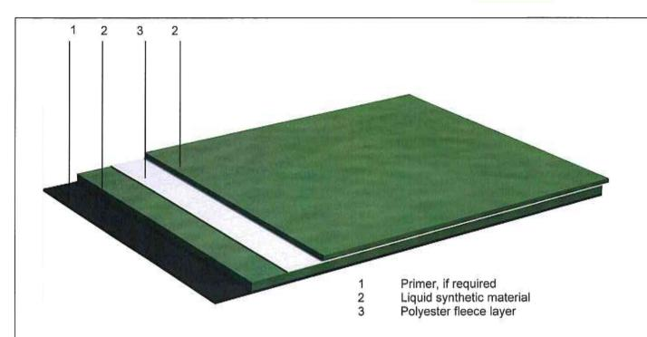
Applicable to the roof waterproofing "Triflex ProTect":
